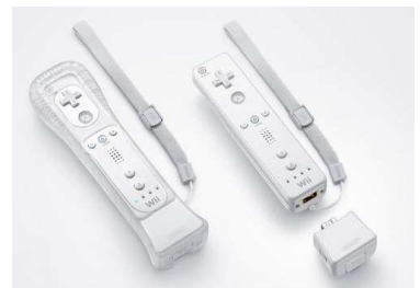
Fig.2 Wii MotionPlus, an expansion device for Wiimote.
